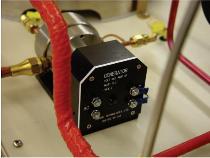
Figure 2.9: AC/DC Electric Generator
